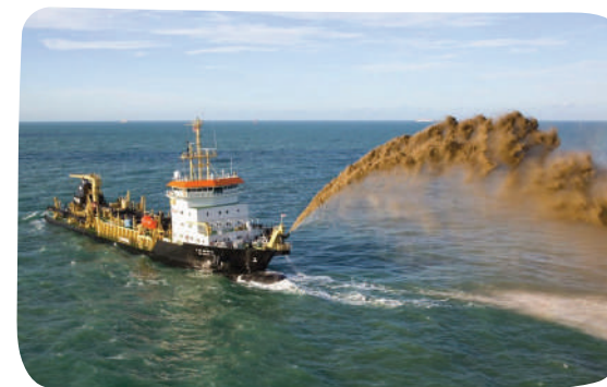
Fig. 12 - A dredging vessel. Dredging is the removal of sediment and other materials from the bottom of a body of water, usually done to keep waterways and ports navigable, as well as for coastal redevelopment.
